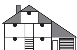
Recommended placing for the Smoke Alarm: 1 smoke detector on each floor.
